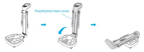
3. Put the InBody into the packing box. Place the packing pad over the equipment and tape up the packing box.
